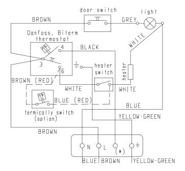
Connector \* is in the junction box market depending on producer of compressor as follows
